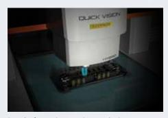
Example of measuring an engine control unit
