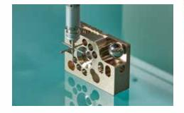
4 Capturing microscopic features of a 3D object using white light interference White Light Interferometer
