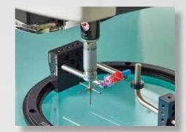
Example of measuring a valve used in medical equipment
